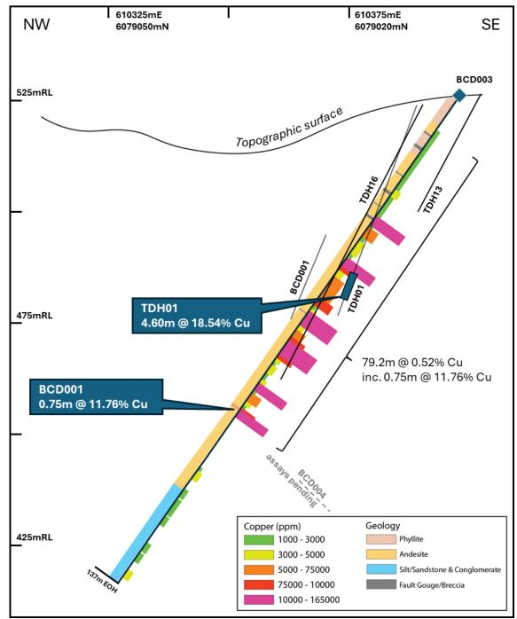
**Figure 1** - Schematic NW-SE cross section (40 metre window, view looking towards the northeast through Section B-B') of the Basin Creek prospect showing diamond drill hole BCD003 with the reported copper assay intervals and historic AOG intercept in TDH01<sup>3</sup>.
