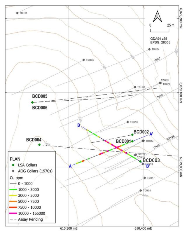
**Figure 3** - Updated locational map of the Basin Creek prospect, showing diamond drill hole collars and drill traces in plan view, with intervals containing recently received copper assay results from BCD001 and BCD003 highlighted. Position of cross sections A-A' and B-B' also shown.
