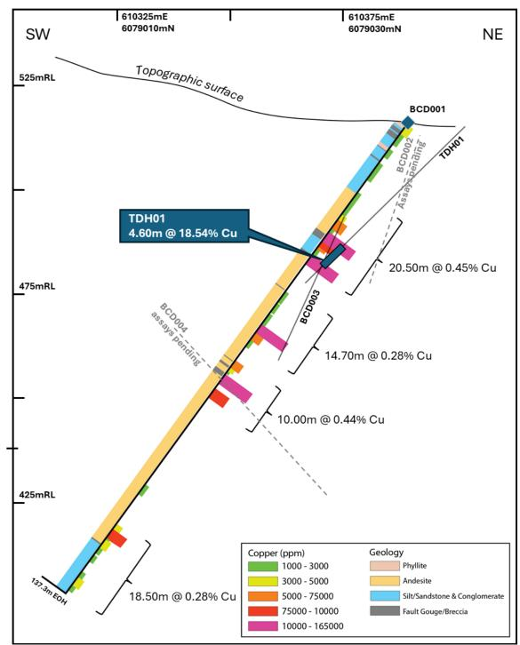
**Figure 2** - Schematic SW-NE cross section (40 metre window, view looking towards the northwest through Section A-A') of the Basin Creek prospect showing diamond drill hole BCD001 with the reported copper assay intervals and historic AOG intercept in TDH01<sup>4</sup>.
