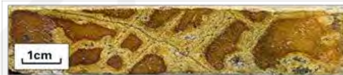
TDH01 4.6 metres at 18.54 % Cu from 57.9 metres 1 massive chalcopyrite (copper sulphide) - tarnished by length of time in core tray
