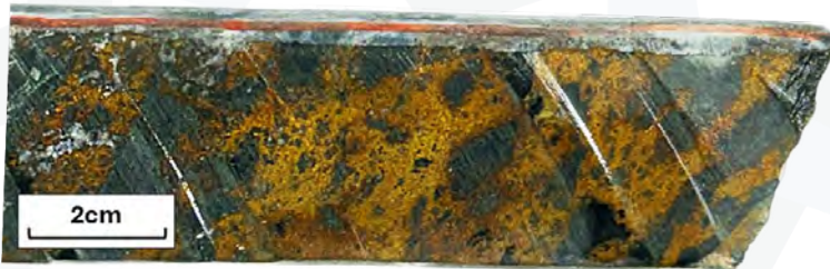
TDH09 1.5 metres at 6.40 % Cu from 205.8 metres 1 chalcopyrite (copper sulphide) in chlorite-magnetite-quartz altered intermediate volcanoclastic breccia. Chalcopyrite tarnished by length of time in core tray
