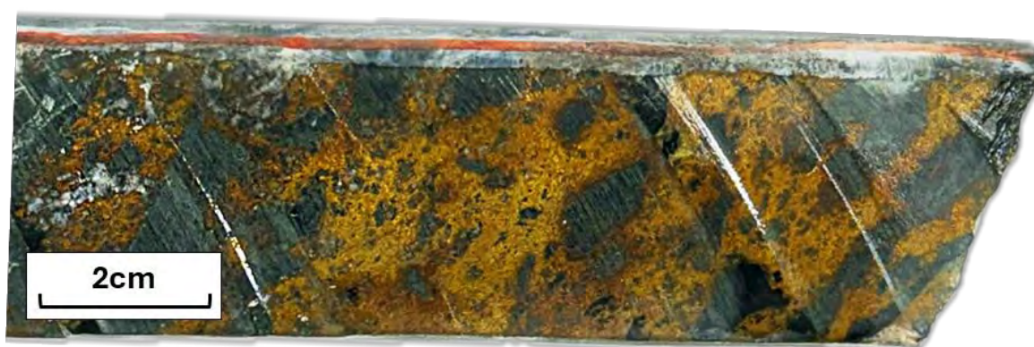
Figure 2: Photo of diamond core completed by Australian Oil & Gas Minerals Pty Ltd (1970's). Sample interval of 1.5 metres at 6.40 % Cu from 205.8 metres in TDH09 1 containing (tarnished) chalcopyrite (copper sulphide) in chlorite-magnetite-quartz altered intermediate volcanoclastic breccia. Core diameter is BQ (36.4mm) with half core retained as a representative sample.
